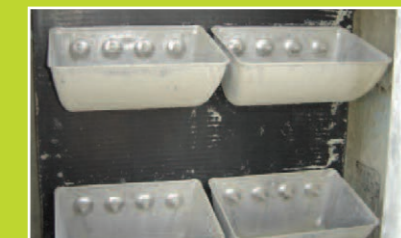
Starco Jumbo Buckets on 4B Steel Web Belt Cement Application
