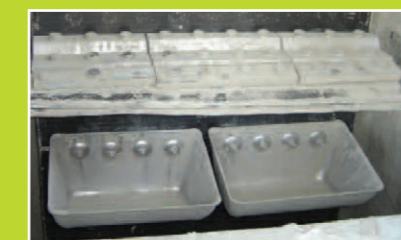
Braime Clamp Belt Splice on 4B Steel Web Core Belt
