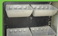
Starco Jumbo (SJ) Buckets on 4B Steel Web Core Belt in Cement Application
