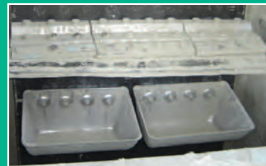
Braime Clamp Belt Splice on 4B Steel Web Core Belt
