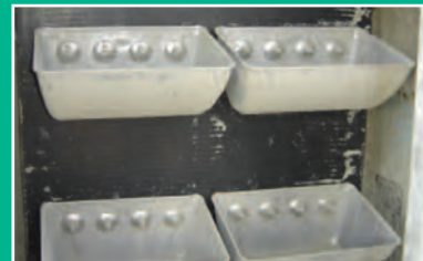
Starco Jumbo Buckets on 4B Steel Web Core Belt Cement Application
