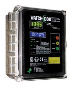
An LCD screen displays elevator status messages (available in four different languages) and a superbright LED screen displays belt speed. RS485 communication is also available for connection to plant computers / PLCs. Calibration and parameter adjustment are all menu-driven and kept simple.
