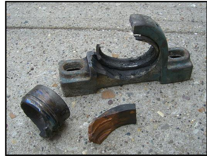
Example of Bearing Failure
