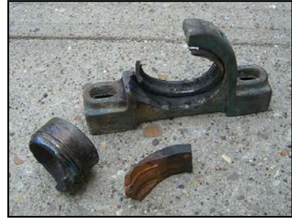
Example of Bearing Failure
