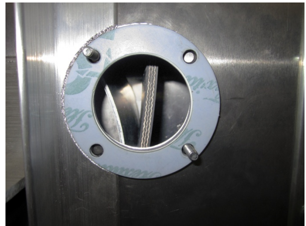
Figure 1 – TouchSwitch Mounting Hole
