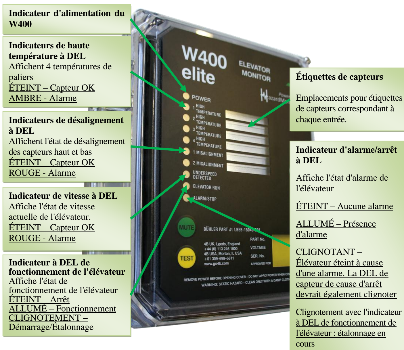
Figure 15 – W400 Controller LEDs
