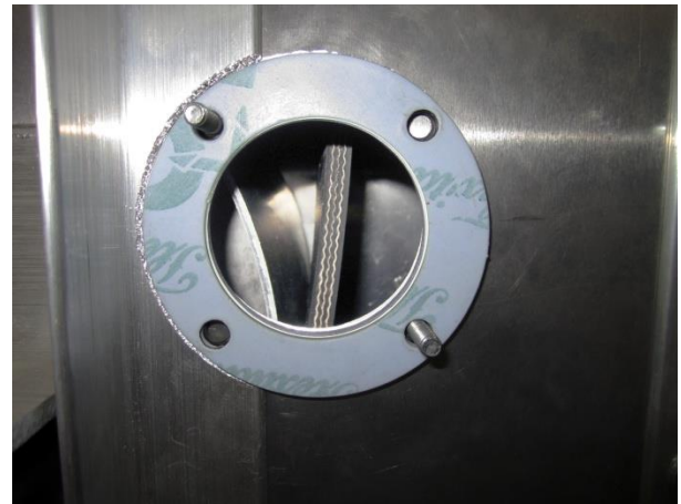
Figure 1 – TouchSwitch Mounting Hole
