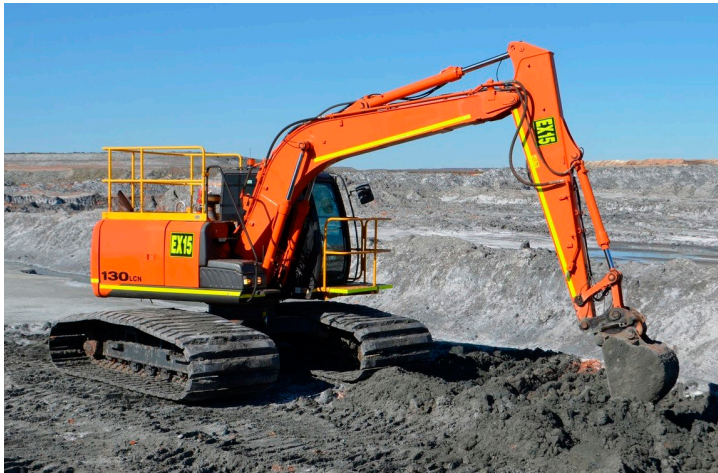
Nylathane™ tractor pads used on an excavator
