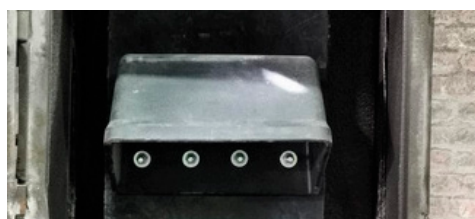
Nylathane™ buckets installed in glass cullet elevator
